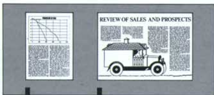
Document width sensing automatically selects the right frame size for you. Filmed images are always upright for easy reading.
