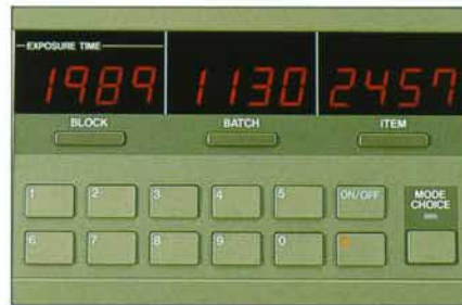
Frames can be precisely identified with frame number, time, date or other information.
